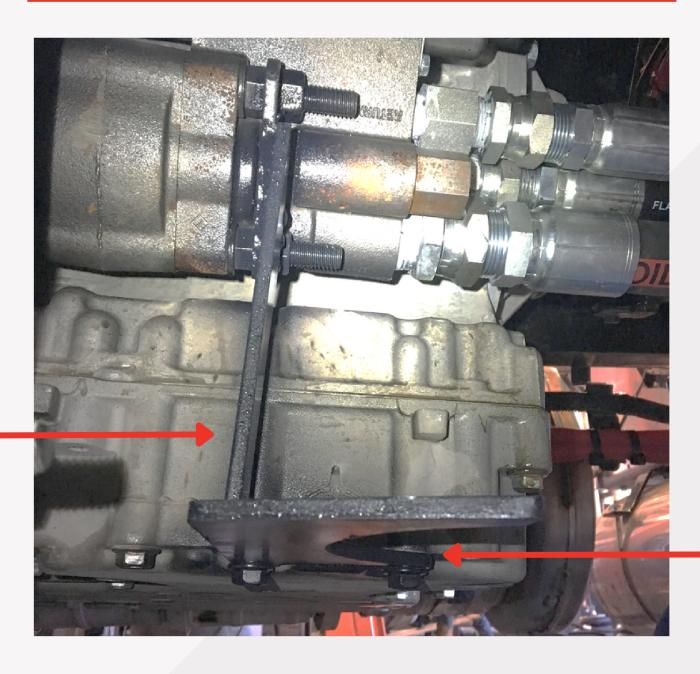
No gussets to prevent flexing at welded corners. Therefore, the bracket will flex as the truck bounces. Bracket is connected to transmission via pan bolts—this is **not** a suitable bracket mounting location.
