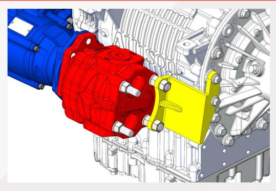
In the example above, the pump support bracket (shown in yellow) meets Muncie Power's design requirements for it to be mounted to the transmission and to the hydraulic pump.
