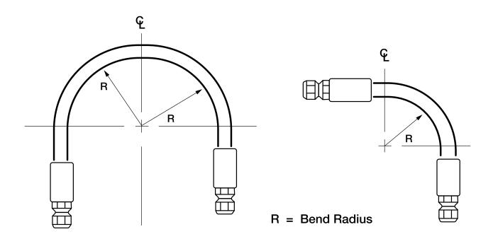
The minimum bend radius is measured from the inside edge of the hose to the centerline of the bend.
